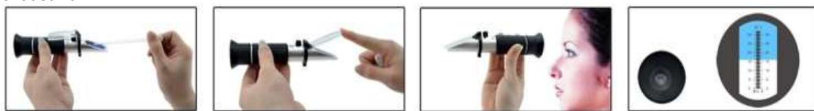
After each use, clean the instrument by using a soft cloth. Don't put it into water since then it might become foggy and useless. The Refractometer is an optical instrument. It requires careful handling and storage. With care, this instrument will provide years of reliable service.
